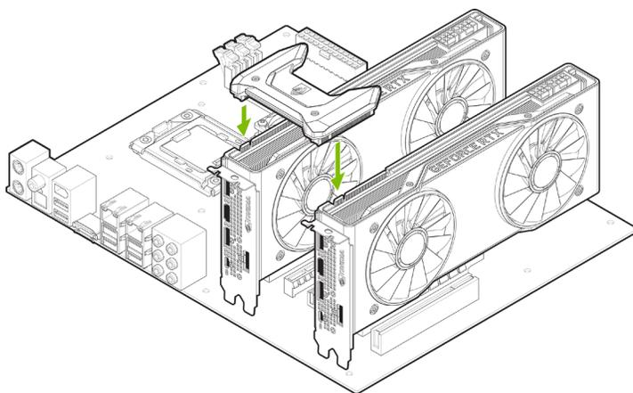
2-way SLI: Install your second GeForce RTX 2080 Ti graphics card into the outer PCI Express x16 slot (the outer slot is the one farthest away from the CPU).
