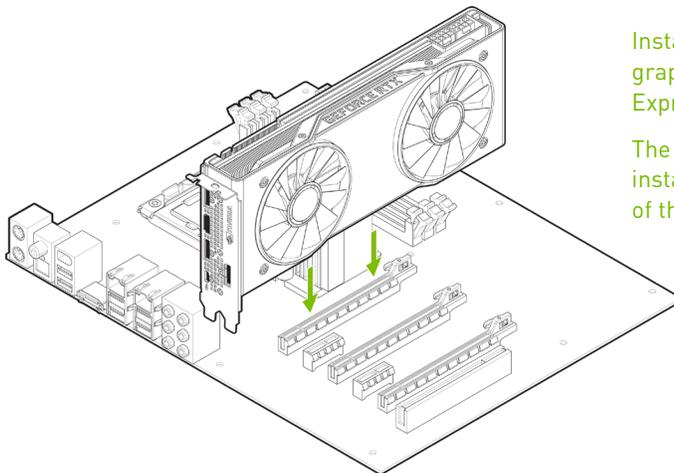
Install your first GeForce RTX 2080 Ti graphics card into the Primary PCI Express x16 slot.
