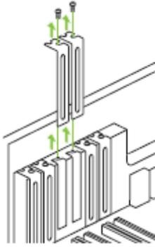
Remove two adjacent slot covers that corresponds to the PCI-Express slot you are installing the GeForce RTX 2080 Ti graphics card in.
