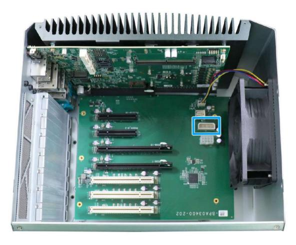
The system's daughter board features a 4-pin connector to supply additional power for users who install add-on PCIe USB3 or Power over Ethernet (PoE) cards that may require extra power delivery.
