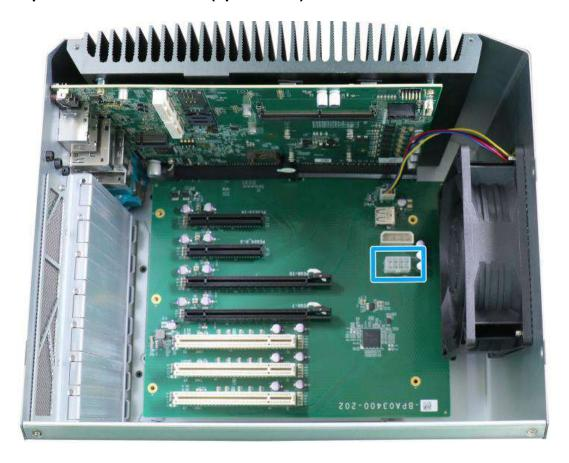
The system supports an NVIDIA graphics inference accelerator up to 115W. The 8-pin connector can supply additional power delivery to the graphics card for operation stability.
