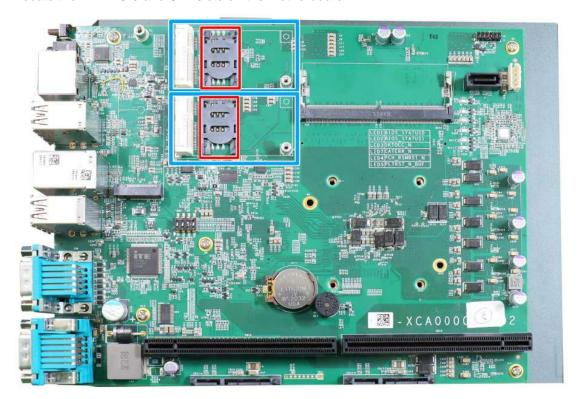
3. Before installing the module, you need to insert the mini-SIM card. Slide the SIM slot holder and lift the SIM card holder. Insert the Mini-SIM card (pins facing up), shut the SIM holder and slide it to lock the SIM card in-place.
