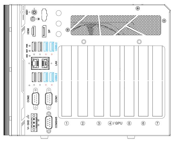
The system's USB 3.2 Gen1x1 ports (5Gbps) feature panel screw fix hole (indicated in **red**), and are implemented via native xHCI (eXtensible Host Controller Interface) controller. They are backward compatible with USB 2.0, USB 1.1 and USB 1.0 devices.
