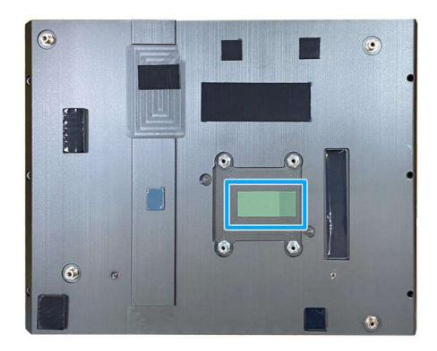
7. Remove and clean off any thermal pad residues around the socket/ motherboard. Gently place the new CPU into the socket by matching the four notches (indicated by blues arrows) on the side to the protrusions in the socket. Pay attention to the seating orientation, notice there is a short side (indicated by green lines), and a long side (indicated by red lines).
