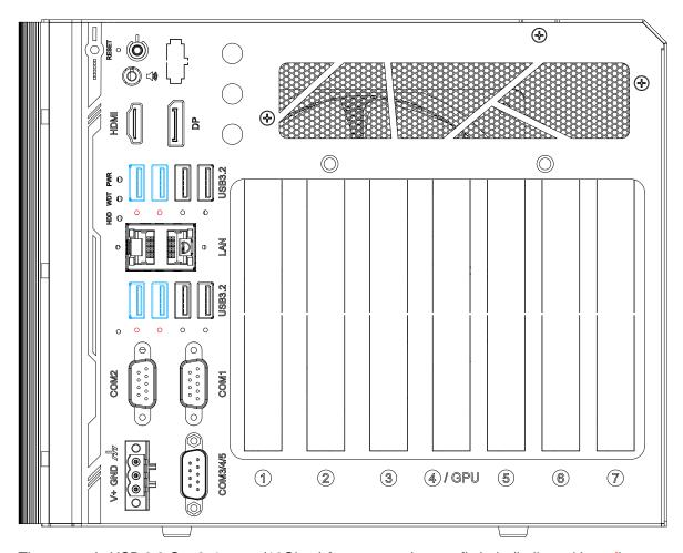
The system's USB 3.2 Gen2x1 ports (10Gbps) feature panel screw fix hole (indicated in red), and are implemented via native xHCI (eXtensible Host Controller Interface) controller. They are backward compatible with USB3.2 Gen.1 USB 2.0, USB 1.1 and USB 1.0 devices. Legacy USB is also supported so you can use USB keyboard/mouse in DOS environment.
