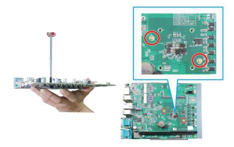
Hold CPU retention bracket firmly and turn the motherboard around
