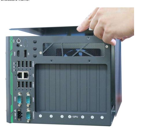
2. Secure the screw indicated on the I/O panel.
