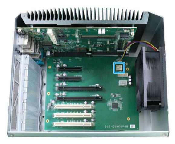
The system's daughter board has an internal USB2.0 port on the PCBA. You can utilize this USB port to connect a USB protection dongle inside the chassis of the system.
