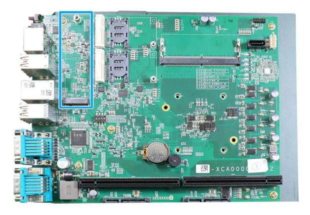
The system has an M.2 2280 slot (SATA signal only) for you to install an M.2 SATA SSD for faster access over traditional hard disk drives.
