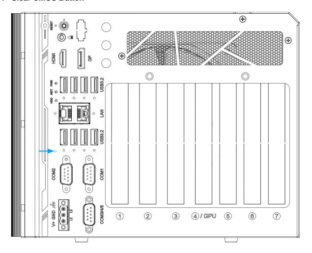
Indicated by the **blue arrow**, the CMOS Reset button is used to manually reset the motherboard BIOS in case of system halt or malfunction. To avoid unexpected operation, it is purposely placed behind the panel. To reset, please use the tip of a pen, press and hold for at least 5 seconds to reset the BIOS.
