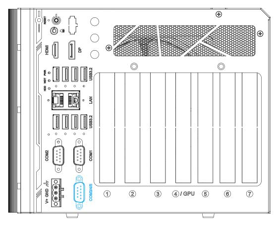
COM3, COM4 and COM5 are 3-wire RS-232 ports share single DB9 connector. You can directly connect this to one external device with 3-wire RS-232 interface, or use an optional 1-to-3 Y-cable to have three DB9 connectors for more devices. The following table describes the pin definition of the DB9 connector as well as the Y-cable.
