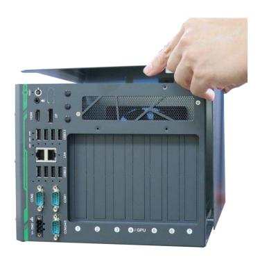
5. Once the L-shaped panel has been removed, you can gain access to all internal expansion slots and components.
