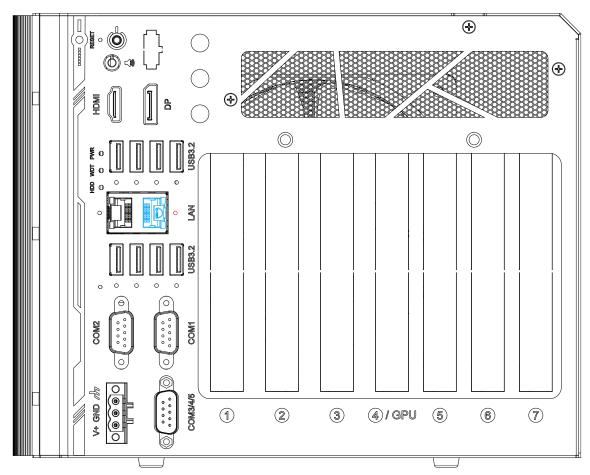
The system has a 2.5Gb Ethernet port featuring panel screw fix hole (indicated in red).
