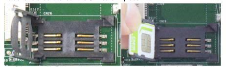
Slide and lift SIM card holder Insert SIM card with pins facing up
