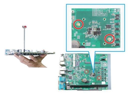
Hold CPU retention bracket firmly and turn the motherboard around
