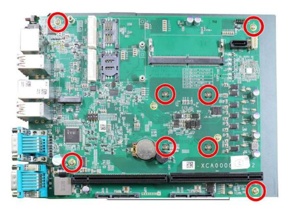
3. Gently separate the motherboard from the heatsink. With a hand on the CPU retention bracket, remove the screws indicated to remove the CPU holder from the CPU.
