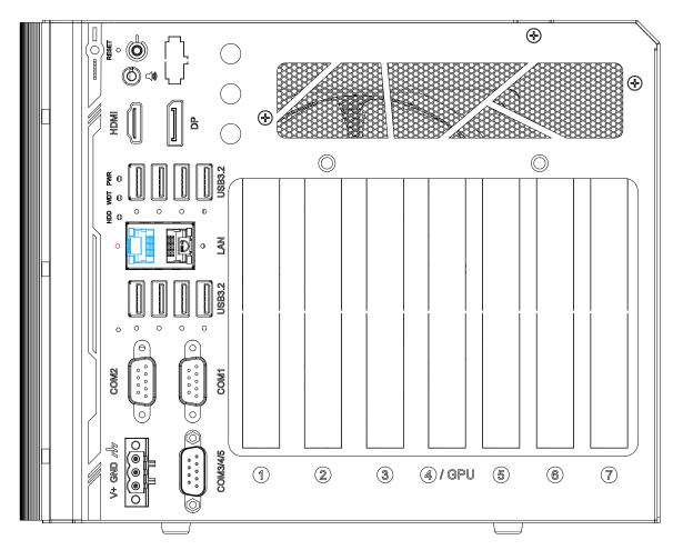
The system has a GbE port featuring panel screw fix hole (indicated in red), and it supports Wake-on-LAN functions. The GbE port is implemented with Intel® I219-LM controller with one dedicated PCI Express link for maximum performance. When the Ethernet connection is established, the LED indicators on the RJ45 connector represents the following connection statuses:
