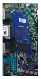
4. Gently press down and secure the module with an M3 P-head screw.
