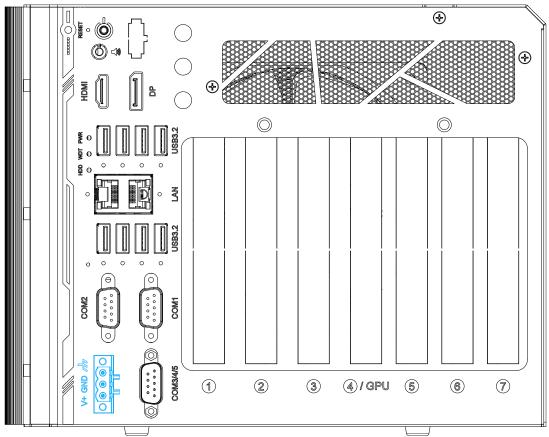
The system accepts a wide range of DC power input from 12 to 35V via 3-pin pluggable terminal block, which is fit for field usage where DC power is provided. And the screw clamping connection of the terminal block gives a very reliable way of wiring DC power.
