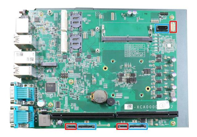
The system provides three SATA ports which support Gen3, 6 Gb/s SATA signals. The SATA ports are indicated in **blue**, and each of their power connectors (indicated in **red**) are situated along side.
