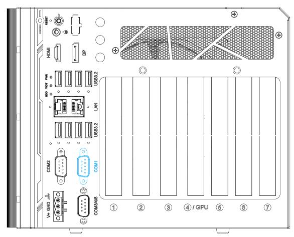
The COM1 port is implemented using industrial-grade ITE8786 Super IO chip (-40 to 85°C) and provide up to 115200 bps baud rate. It is a software-configurable RS-232/422/485 port. The operation mode of can be set in BIOS setup utility. The following table describes the pin definition of the COM port.
