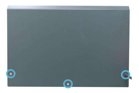
4. Secure the screw indicated at the rear to complete the enclosure installation.
