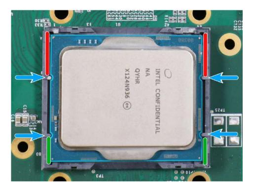
10. Locate the CPU retention bracket (holder) from the accessory box. Place the retention bracket on the CPU and hold it in place. Make sure the screw holes match the CPU retention bracket's screw holes (indicated by red circles).
