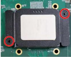
Screw holes for CPU retention bracket
