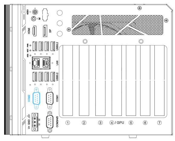
The COM port is implemented using industrial-grade ITE8786 Super IO chip (-40 to 85°C) and provide up to 115200 bps baud rate. It is a software-configurable RS-232/422/485 port. The operation mode of can be set in BIOS setup utility. The following table describes the pin definition of the COM port.
