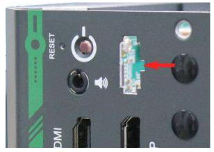
6. Push the plug inside-out, make sure it is clipped onto the I/O panel to complete the optional cable installation.
