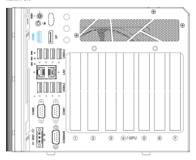
The High-Definition Multimedia Interface (HDMI) port provides uncompressed high-quality digital video and audio transmission between the system and a multimedia display device on a single cable. You can connect to other digital inputs by using a HDMI-to-DVI or HDMI-to-DP cable.
